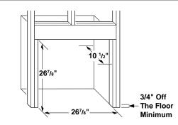
Figure 6 - Rough Opening for Installing in Wall
